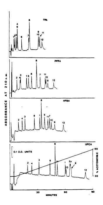
procedure, the compound of interest is contained in a relatively large volume of solvent. This is a distinct disadvantage when isolating peptides in microgram quantities. The properties of other perfluorinated carboxylic acids have been evaluated in order to investigate the possibility that they might introduce a different chromatographic principle into the peptide hormone isolation procedure.
